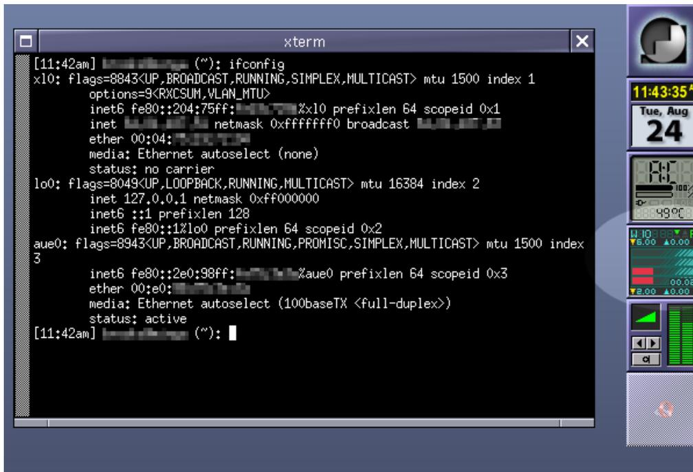
Figure 1: The xterm shows the correct interface listing, but `wmnd` shows `wi0` which has been removed and replaced with `aue0`.
